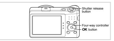
Press the four-way controller (A) in mode. The [Drive Mode] screen appears.
